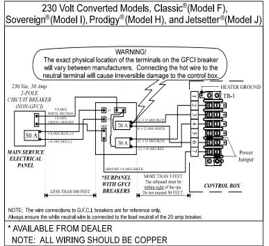
Route the electrical service from the subpanel into the spa equipment compartment. Position the conduit in the recess provided between the frame and the door.
