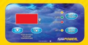
Touchpad fitted to spa pool provides control of pump, blower, second pump and light at your fingertips.
