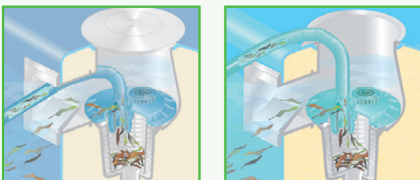
Two options of connecting the hose to the Vacuum Plate Assembly.
