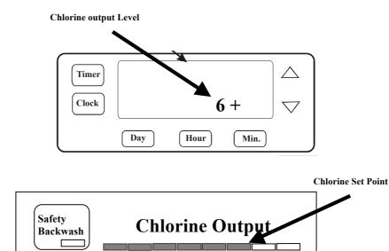
Your VX Salt chlorinator will always attempt to adjust the output so that the actual output level matches set point level. At times when the Chlorine output level is lower than the set point, check the salt level in your swimming pool at your local pool shop. Alternatively, you may have a low voltage supply to the chlorinator (less than 240Volts) or the water may be colder than usual.
