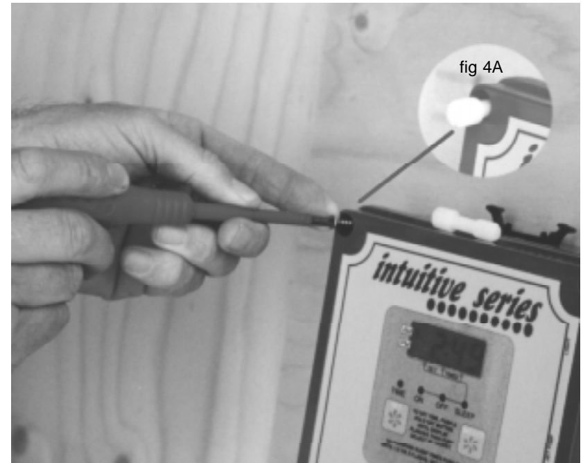
fig 4: Mounting method for control box.
