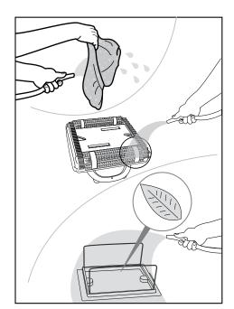
• Refit the filter bag with the tag on the outside positioned centrally along the length side of the bottom lid.
